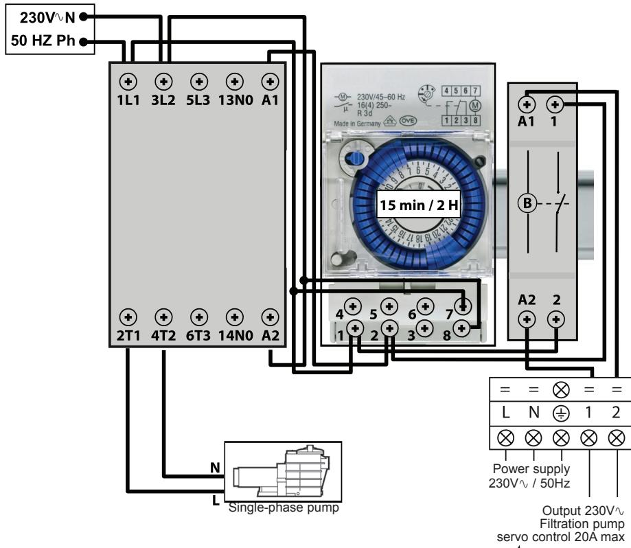
Outside the filtration range, the water temperature needs to be checked by the regular starting of the filtration pump (15 minutes every 2 hours). If the heat pump is needed during this checking period, it will start up and retain the heating priority.
