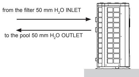
Install by-pass valve between the inlet and outlet on the heat pump.
